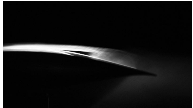
Fig. 19 Flow visualization of the B1.5 model at Re=70000 , \alpha = 3^\circ .
