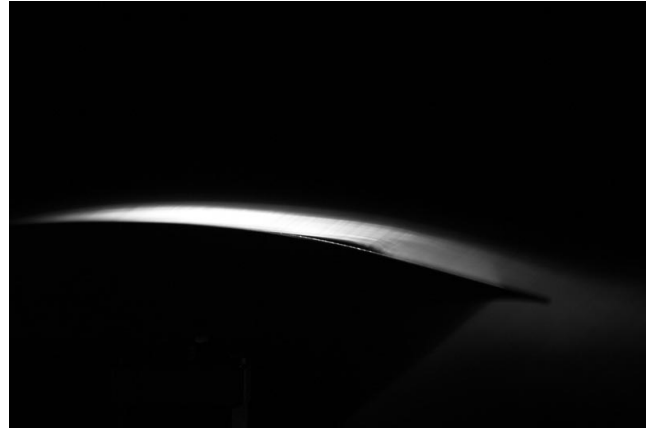
Fig. 18 Flow visualization of the B1.5 model at Re=140000 , \alpha = 3^\circ .
