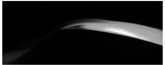
Fig. 11 Flow visualization of the B1.5 model at stall angle. Note the laminar separation bubble near the leading edge.
