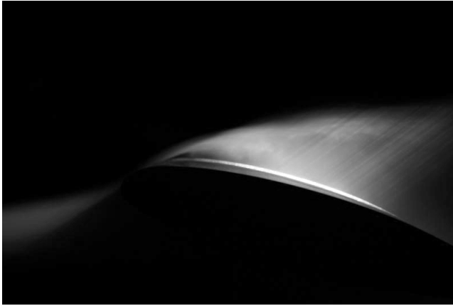
Fig. 12 Flow visualization of the B1.5 model, one degree after stall angle. Note the flow completely separated.
